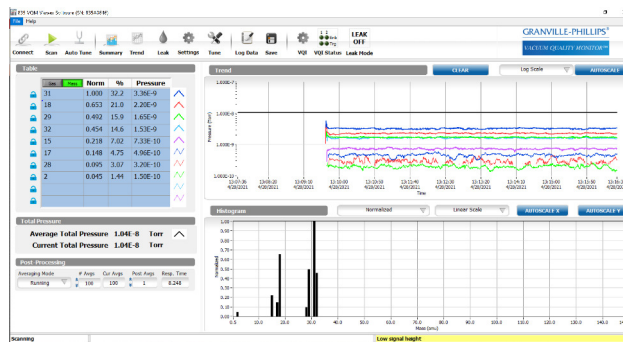
Figure 8: Gases and contamination in the system monitored by a VQM.
