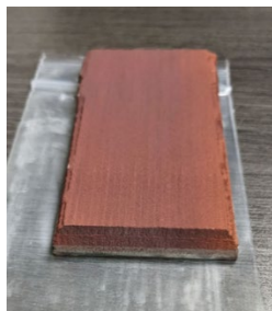
Figure 3: Picture of W40Cu deposited on a Nb sample by cold spray.
