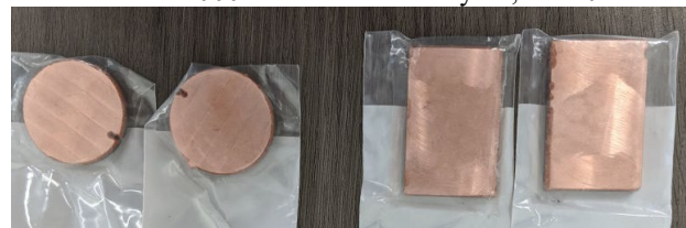
Figure 1: Picture of Nb coupons with 3 mm Cu deposited by cold spray.
