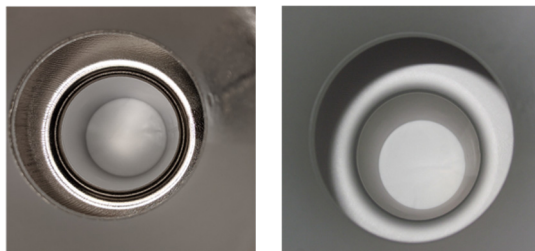
Figure 7: Inside the twin axis cavity #1 before (left) and after the coating (right) [11].
