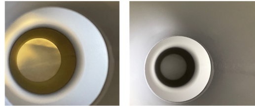
Figure 15: Inside the twin axis cavity #2 after the coating.
