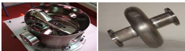
Figure 25: Left: Niobium SSR1 resonator built by IUAC. The photograph shows the interior of the resonator just before its completion. Right: LB 650 cavity developed by VECC in collaboration with IUAC.
