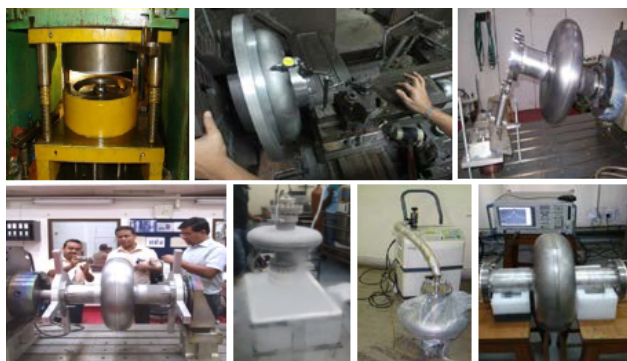
Figure 18: LB single-cell development photos from top left: showing forming, machining, RF measurements, EBW, cryo-shock, MSLD and final RF measurements.
