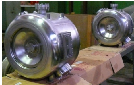
Figure 11: SSR 1 cavities after dressing at BARC.
