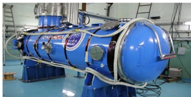
Figure 8: Horizontal test stand developed and commissioned at RRCAT. Magnetic shielding has also been developed and installed.
