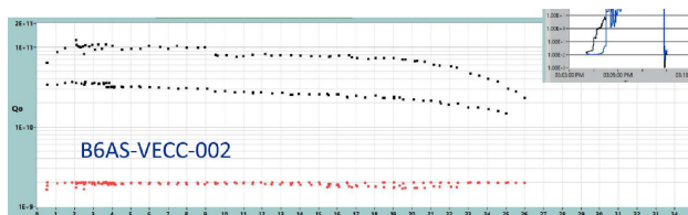
Figure 21: Test results of the second single cell cavity developed by VECC/IUAC.
