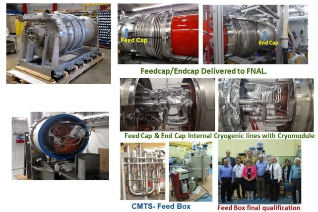
Figure 14: Feed cap and end cap developed by BARC.
