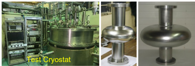
Figure 24: Left Test cryostat, right 1.3 GHz and 650 MHz single cell cavities developed in collaboration with RRCAT.
