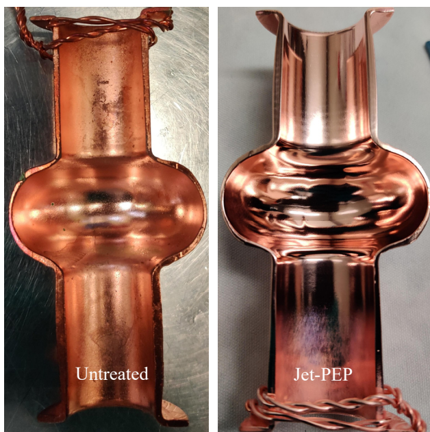
Figure 15: 6 GHz half-cell treated by PEP jet polishing. On the left the cavity before the treatment, on the right the cavity after PEP jet-polishing.
