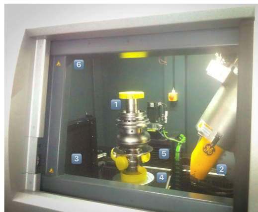
Figure 1: Gun1.1-cavity (1, [4]) placed in between a 300 keV X-ray tube (2) and a detector array (3) on a rotating (4) and lifting (5) table in a shielded cabinet with a lead glass window (6) at XRAY-LAB, Sachsenheim, Germany.
