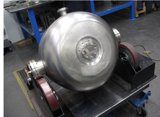
Figure 1: SSR1 SC Cavity Design.
