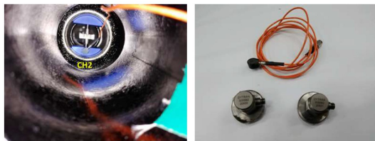
Figure 12: Sensor Fixture and Vibration Sensor.
