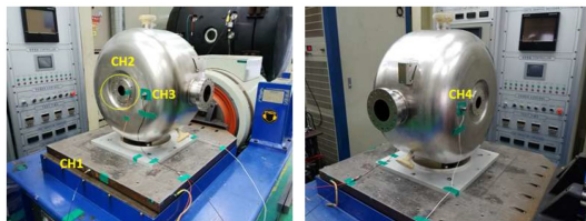
Figure 11: SSR1 SC Cavity Vibration Test Setup.
