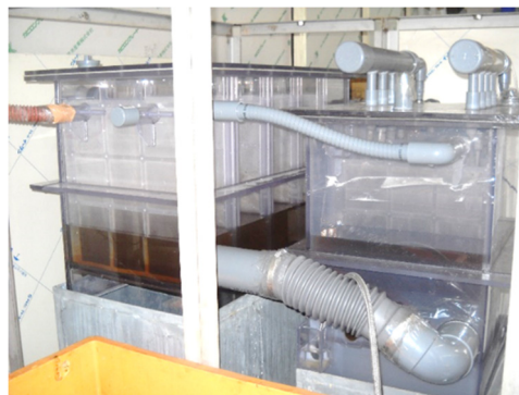
Figure 3: Improved EP acid tank.
