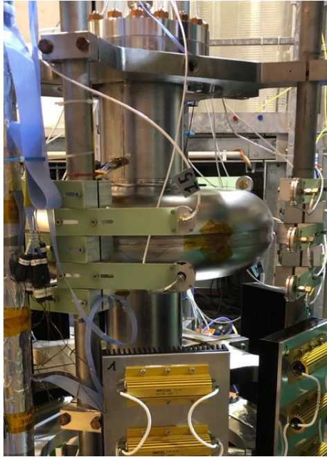
Figure 2: INFN B61S_EZ_001 LB650 cavity installed on the LASA vertical insert before the cold-test. Second sound and temperature sensors are visible around the cell.
