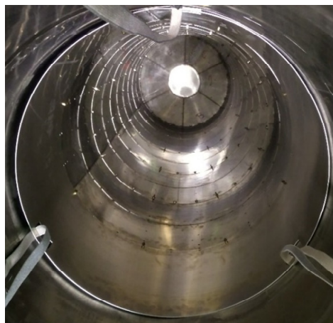
Figure 6: Cryoperm© magnetic shielding in place inside the vertical testing cryostat. A second, external shield at room temperature is placed (not visible here) around the cryostat.
