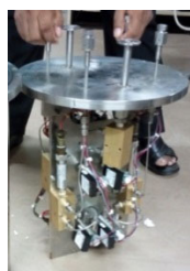
Figure 15: (a) Helium mass flow system; (b) PWM based tuner controller.
