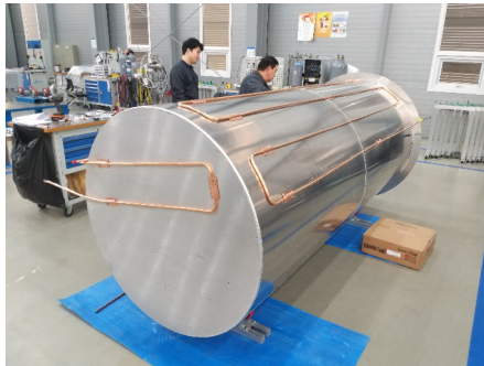
Figure 7: Cryostat thermal shield fabrication.
