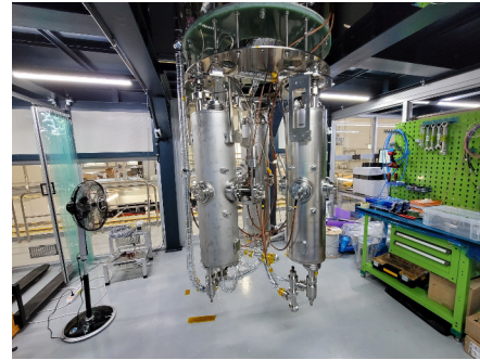
Figure 10: HWR dressed cavity installation for VT.
