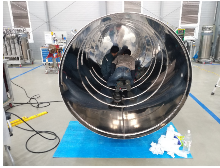
Figure 6: Cryostat fabrication - GTAW process.
