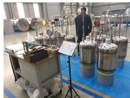
Figure 5: 4K/2K LHe reservoir pressure test with KGS.
