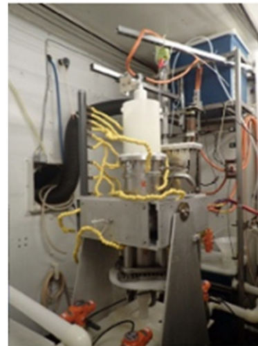
Figure 2: Photograph of the EP of the Cornell B-cell cavity.
