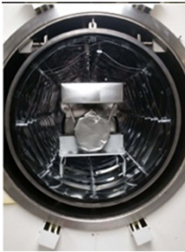
Figure 3: Photograph of the Cornell TM-furnace with the B-cell placed inside.
