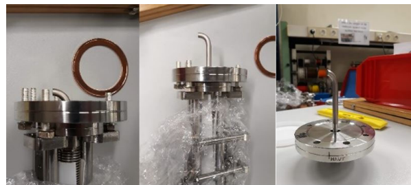
Figure 4: From left to right: Unity coupler fully out, fully in and pick-up antenna.
