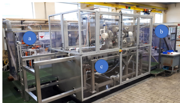
Figure 2: a) copper chemical plant; b) niobium chemical plant; c) cavity handling device.
