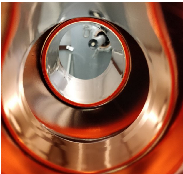
Figure 11: 1.3 GHz copper cavity after electropolishing.
