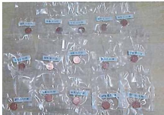
Figure 7: Coupon Cu disks packed in plastic bags after surface-treatment.
