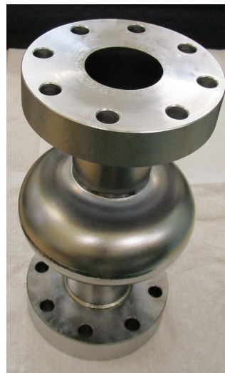
Figure 9: A picture of 3-GHz single-cell Nb cavity with flanges of low-RRR Nb.
