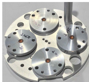
Figure 2: Four coil plates on a base plate.
