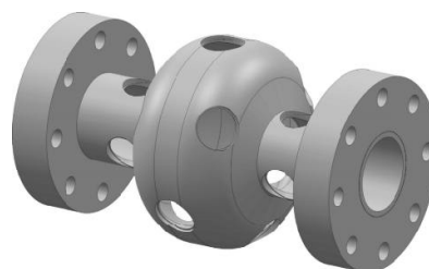
Figure 4: The 3D schematic view of the 3.0-GHz single-cell coupon cavity.
