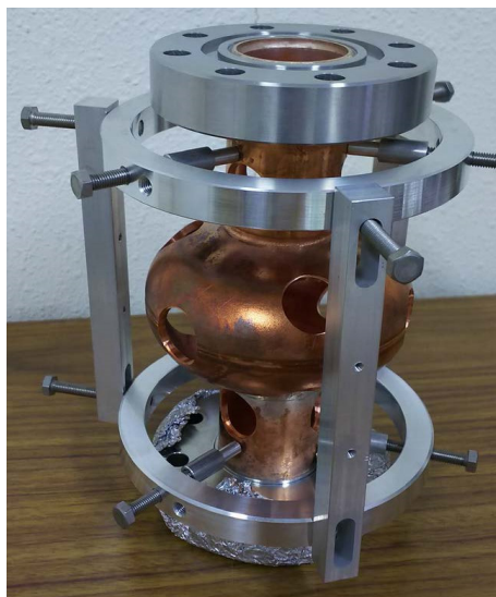
Figure 8: A picture of a coupon Cu cavity with coupon-fixtured.
