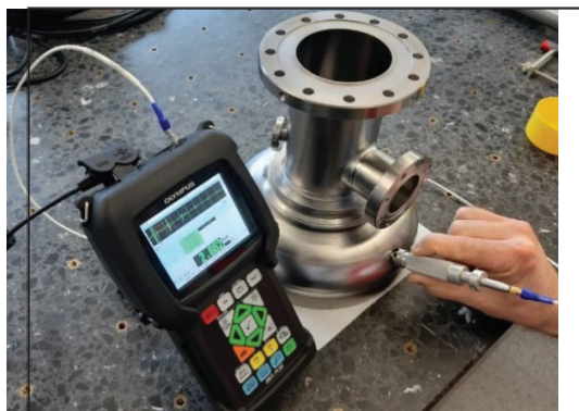
Figure 3: Ultrasonic wall thickness measurement device.
