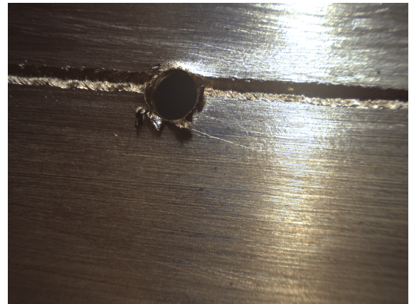
Figure 8: Image of weld seams of a copper 704 MHz 5-cells elliptical test cavity. The image shows details of a drilled 5mm through hole demonstrate the achievable field of view. Lighting for this image was located on the main robotic arm, and the non-uniformity across the image is apparent.
