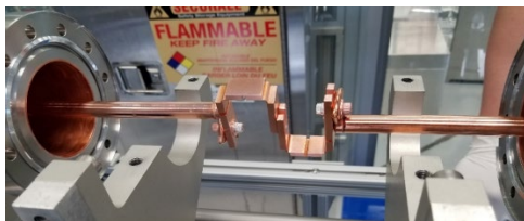
Figure 4: Antenna connection with copper bridge.
