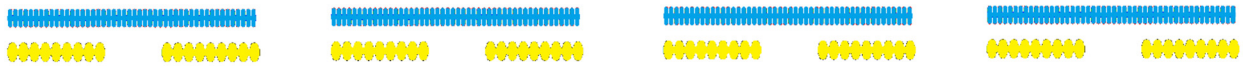
Figure 6: Removing nonaccelerating intervals between cavities: comparison with the TESLA cryomodule comprising 8 cavities.
