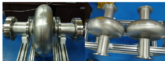
Figure 7: Single cell niobium prototype cavities with stainless steel flanges (left) and niobium flanges (right).
