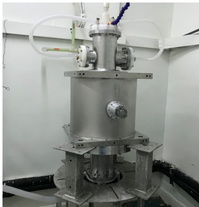
Figure 7: BCP of outer surface (up) and inner surface (down).
