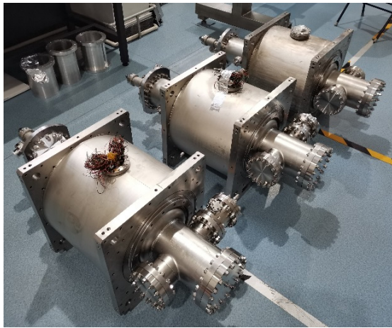
Figure 6: 650 MHz 2-cell cavities jacketed.
