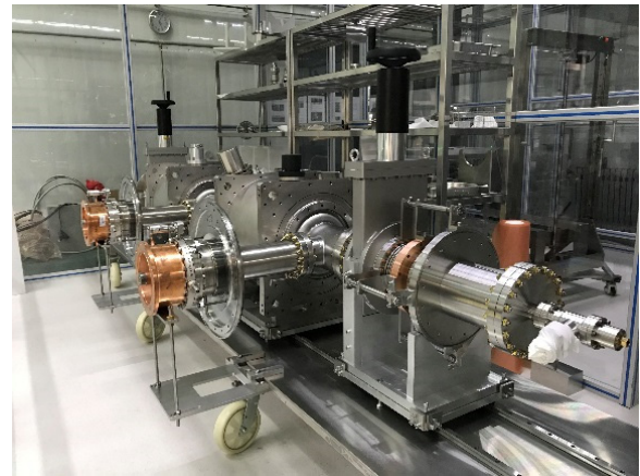
Figure 8: cavity string in cleanroom.
