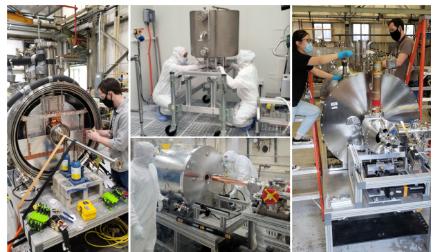
Figure 3: Photos of disassembly, cleaning, and reassembly of the WiFEL cryostat. Initial disassembly (left), high pressure rinsing the cavity (middle, top), cleanroom assembly (middle, bottom), and cryostat assembly (right).
