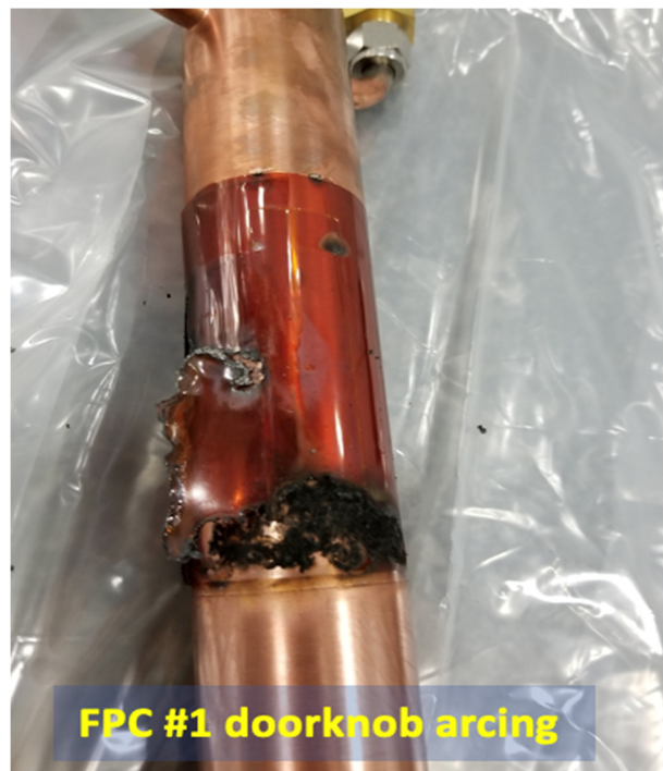
Figure 5: Arc mark in the FPC#1 airside.
