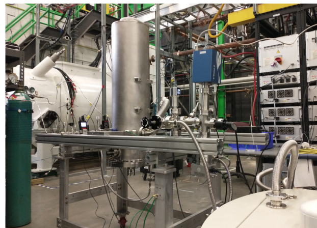
Figure 14: Bench plasma cleaning of a \beta = 0.085 QWR.
