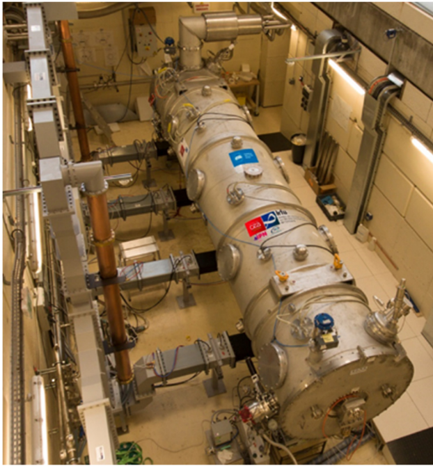
Figure 2: Medium beta cryomodule (CMM) installed in the test stand at CEA Saclay.
