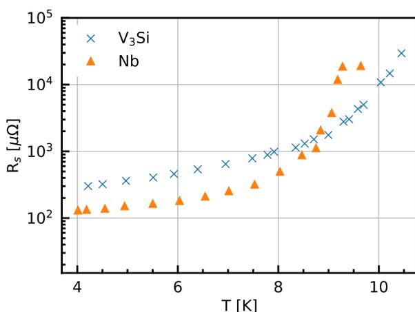
Figure 4: The surface resistance as a function of temperature for the Nb and  $V_3Si$  coated split cavity.
