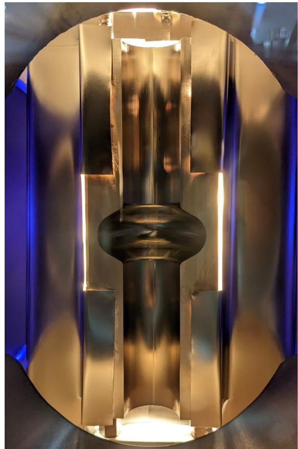
Figure 3: Split 6 GHz cavity during deposition with each half of the cavity deposited sequentially.
