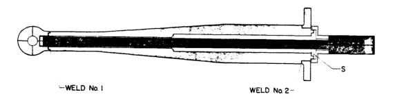
beam welder and allows the internal plate to stub weld to be done before any external welding. This assures a strong joint. The weld chosen penetrates 1.7 mm as opposed to the 1 mm possible in the previous design. A similar weld joins the stub to donut and this too is accomplished with the draw bar keeping the joint under compression. Evidence of this compression is that the finished weld is convex. This greatly simplifies polishing.
