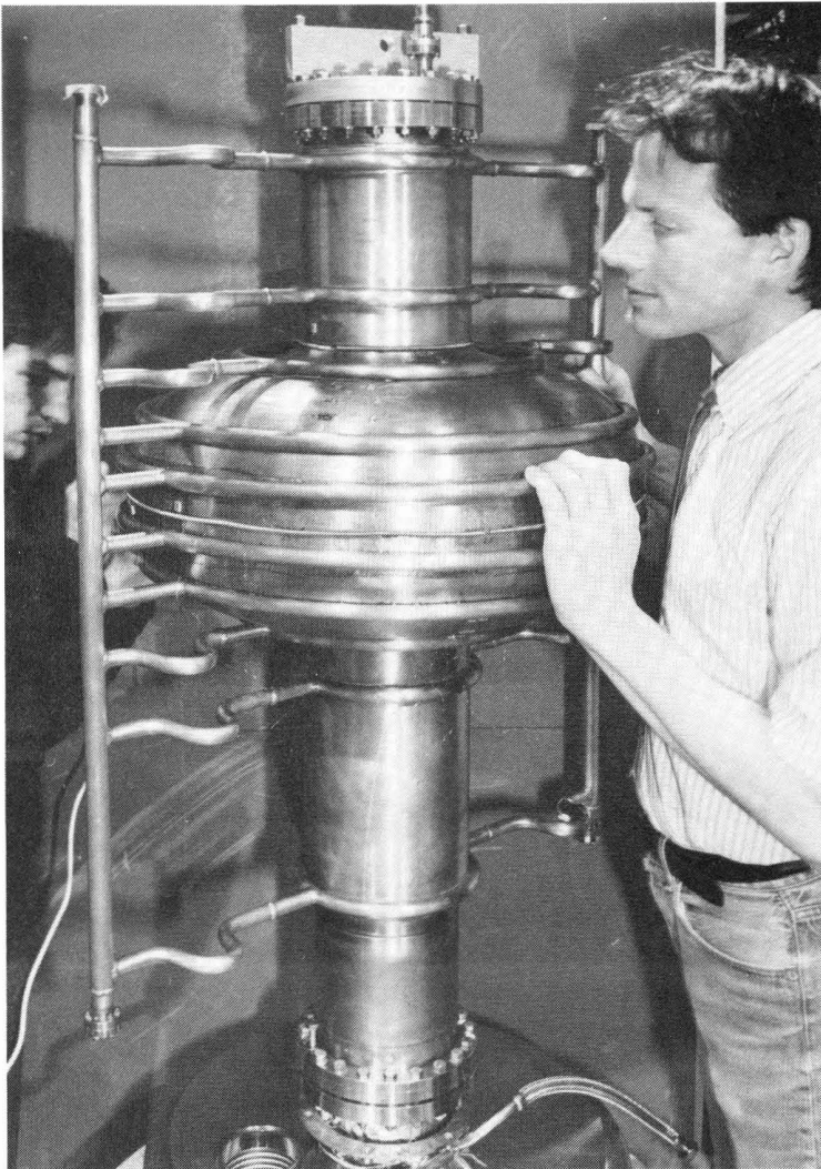
Fig. 3 Pipe cooling version of a 1 cell cavity
