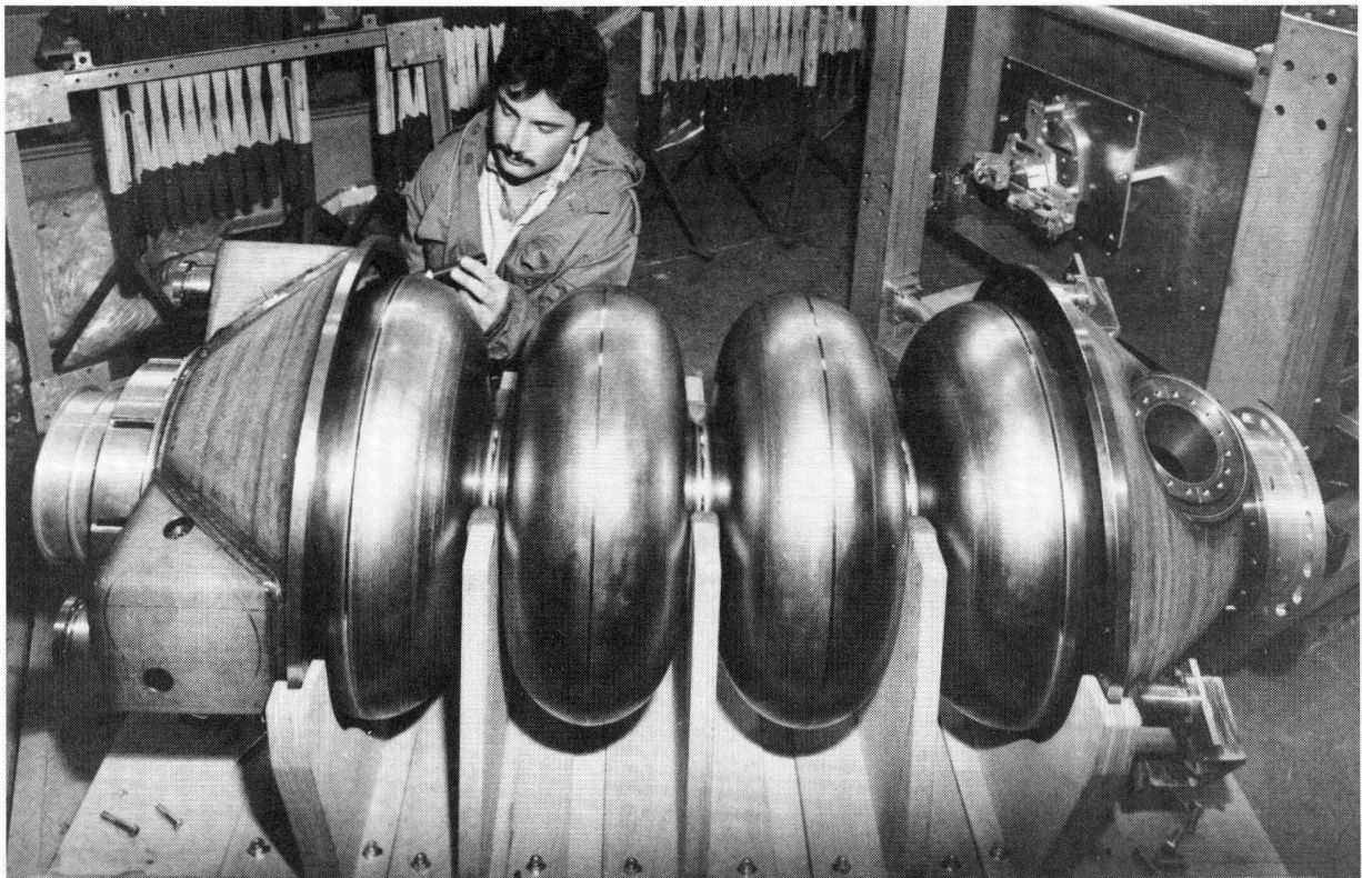
Fig. 6 4-cell Nb-cavity before closing the LHe container
